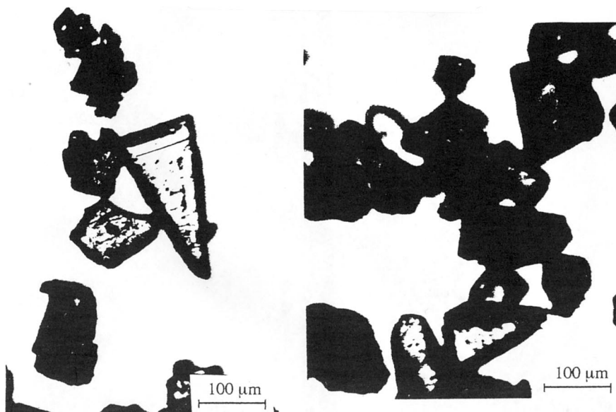
Fig. 5. Appearance of lactose crystals under optical microscope. Left: native crystals; right: ground crystals.
